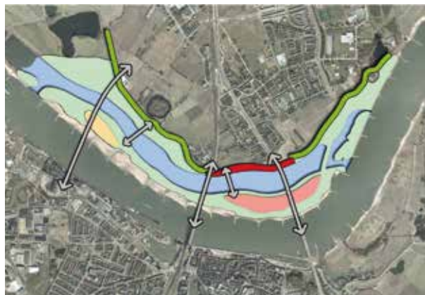
Figure 2: The 'Room for the River' plan at Nijmegen. The green line indicates the current line of the protective dike. The red line shows the position of the proposed relocated portion of dike. In the bottom image, the new river channel is shown in blue and the new island in yellow/green. The white arrows represent the bridge connections planned for the island.
