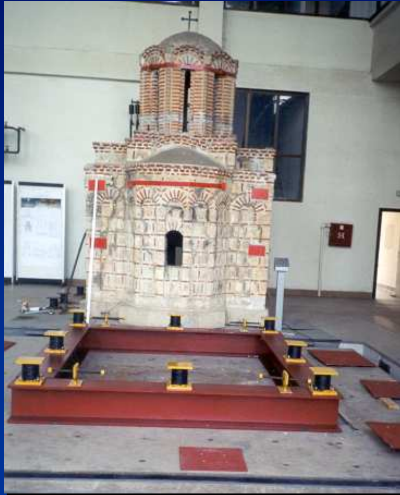
Steel structure and Isolators
