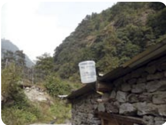
Figure 3.8: Rain Gauge at Timbu, Upstream of Melamchi River, Nepal
