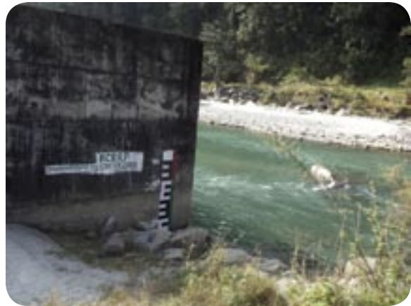
Figure 3.9: River Water Level Gauge in Dolakha, Nepal
