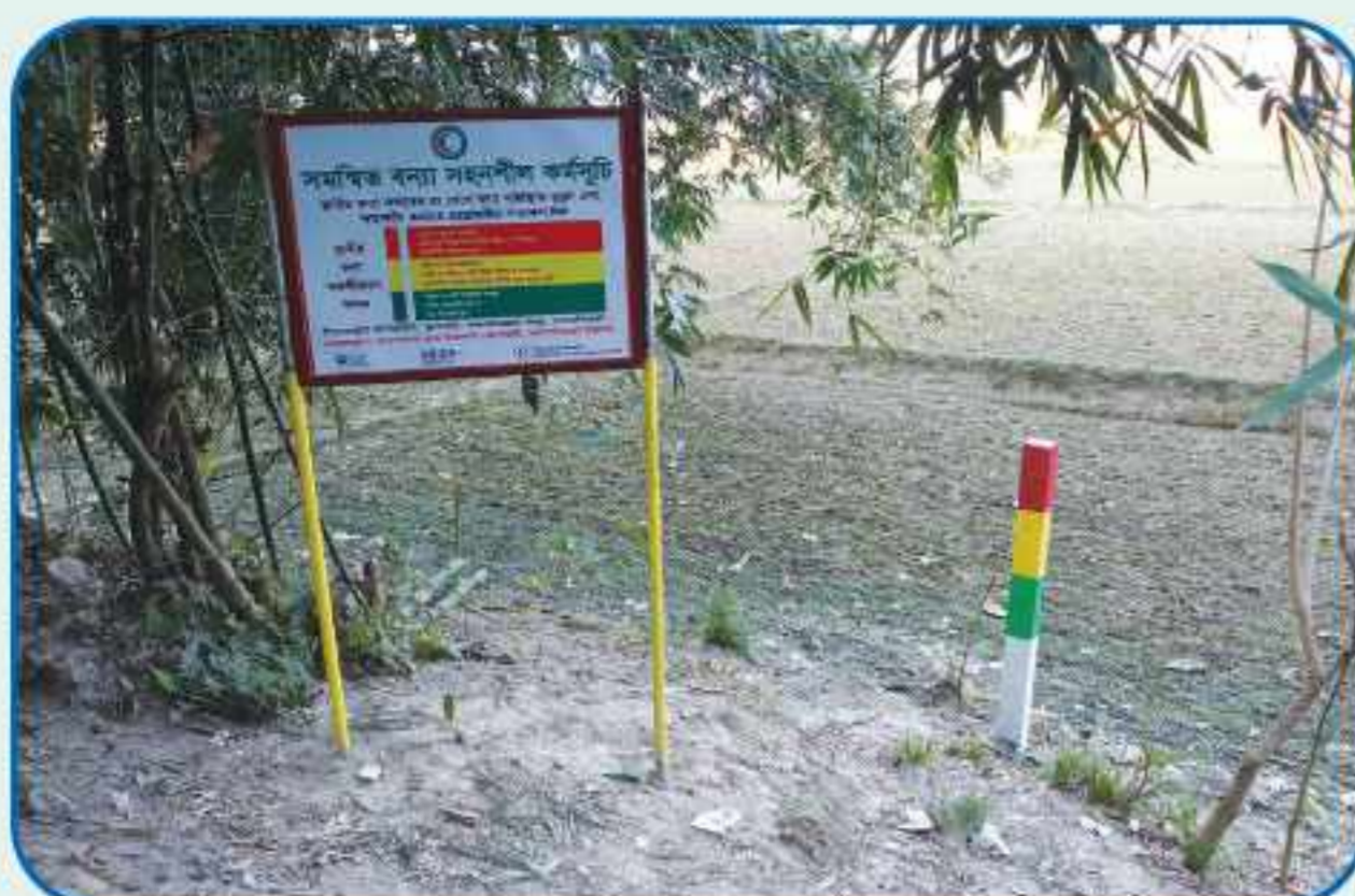
Flood marker with explanatory signboard beside the Dharla river, Shiber Kuti community, Lalmonirhat (Photo: IFRC)
