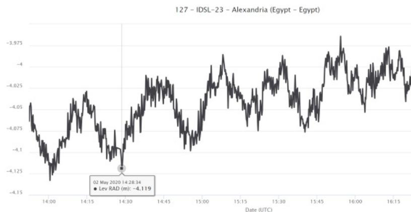
Figure 7. Tsunami record at Alexandria station.
