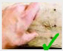
leave a mark (Soft wood) When pressed by tip of nail doesn't leave a mark (Hard wood)
