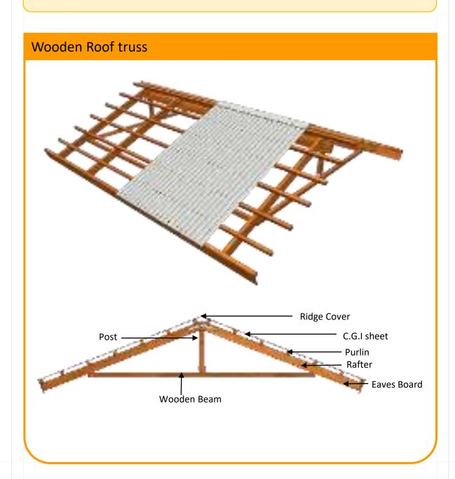
A **timber roof truss** is a structural framework of timbers designed to bridge the space above a room and to provide support for a roof. Trusses usually occur at regular intervals, linked by longitudinal timbers such as purlins.
