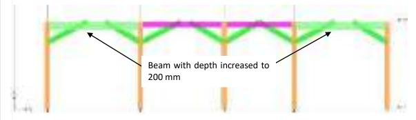
Figure 6: Beams with depth increased to 200 mm
