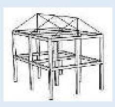
Rigid frame system also known as "Bare timber Frame" is an unbraced frame, that is capable of resisting both vertical and lateral load by the bendings of beams and columns. It is a rectilinear assemblage of beams and columns, with rigid connection between column and beam.
