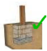
Excavate the soil around the column and construct stone/brick masonry.
