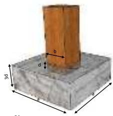
a= 3b or greaterd=b/3 or 50mm, whichever is maximumb= size of column
