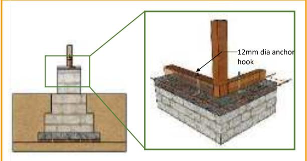
Connection details of wooden Plinth band and column
