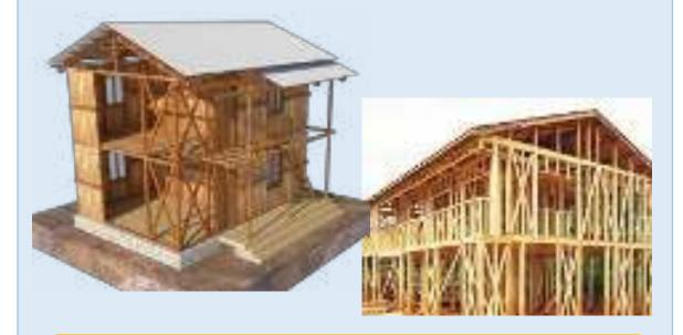
Required brace / shear panel member should be calculated. Simplified calculation method is introduced in this manual.
