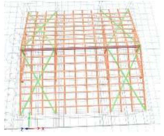
Figure 5: Diagonal Roof Bracing
