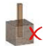
Timber column is embedded in soil only
