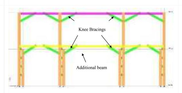
Figure 2: Additional beam above the level of existing beam
