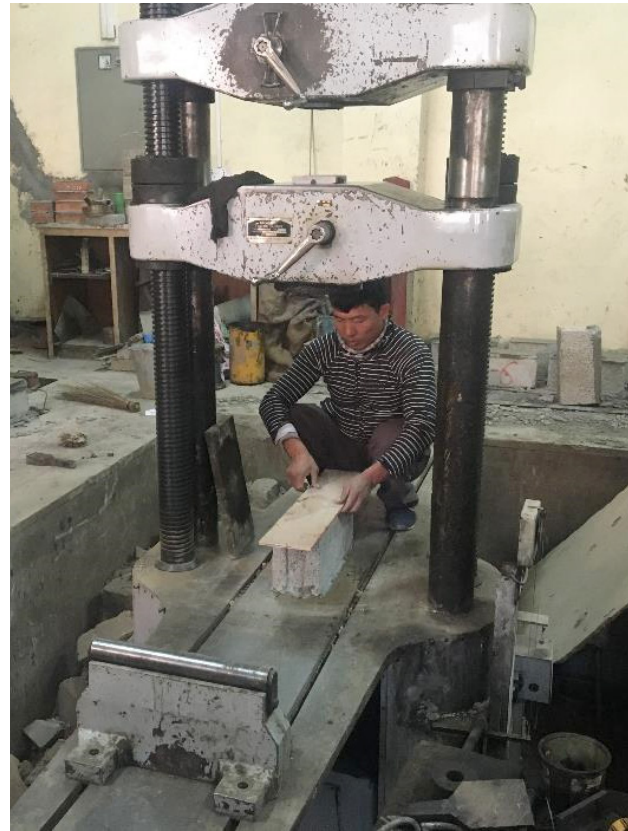
Block testing in the central material testing laboratory, IoE.
