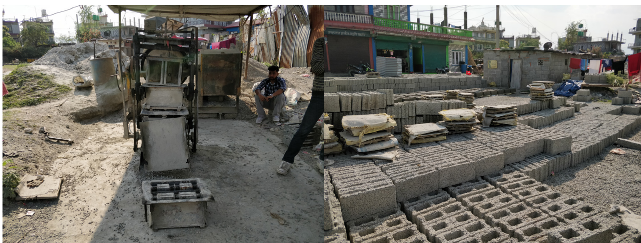
Lekhnath Municipality, Pokhara, Kaski: hollow concrete block production at 'Pokhara Block Udhog'. They produce 30 blocks from one bag of cement, and blocks cost between 40 and 60 NPRs per piece depending on the quality. They produce a maximum of 400 blocks per day.
