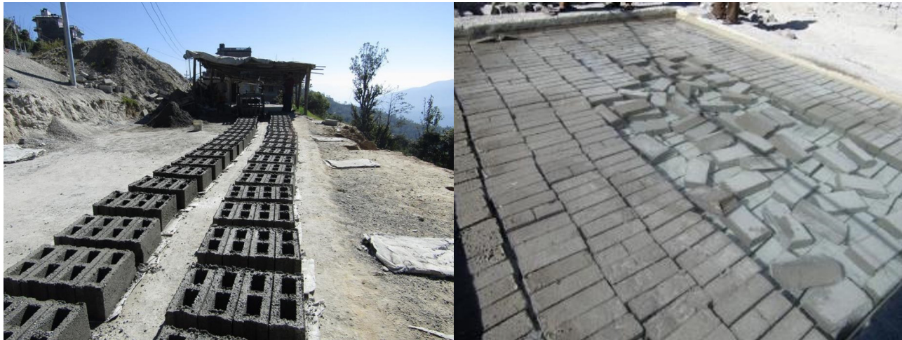
Blocks are laid in the sun after production in Dolakha (L) and blocks submerged in a pond in Dolakha (R).
