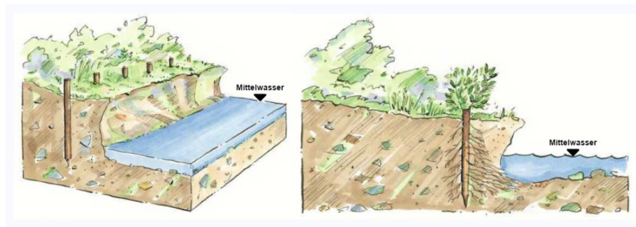
Embankment stabilization by stem sets (Jany & Geitz, 2013)
