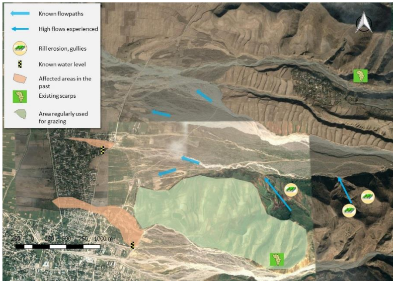
Figure 12: Example of a simple flood inventory map based on knowledge from past events
