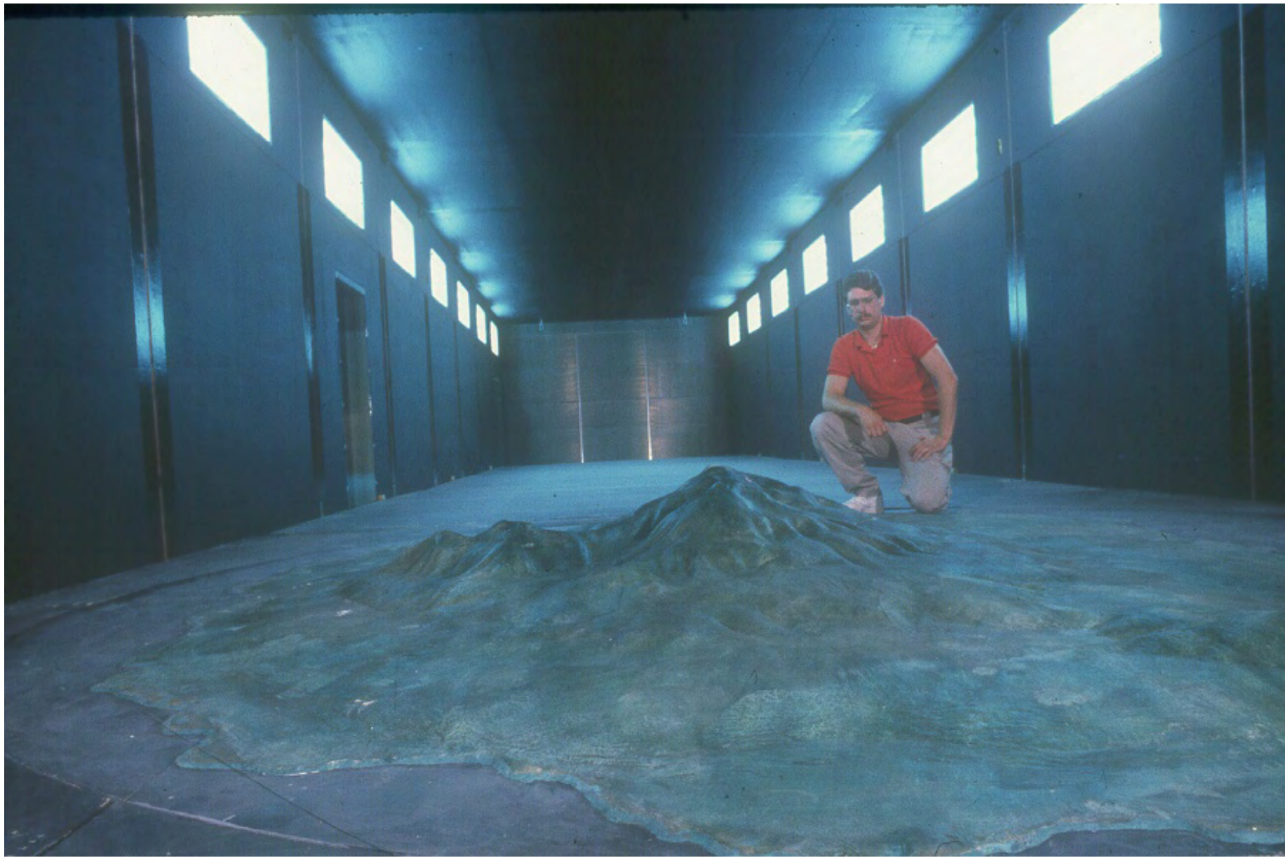
Nevis tested at the Boundary Layer Wind Tunnel Laboratory (UWO)
