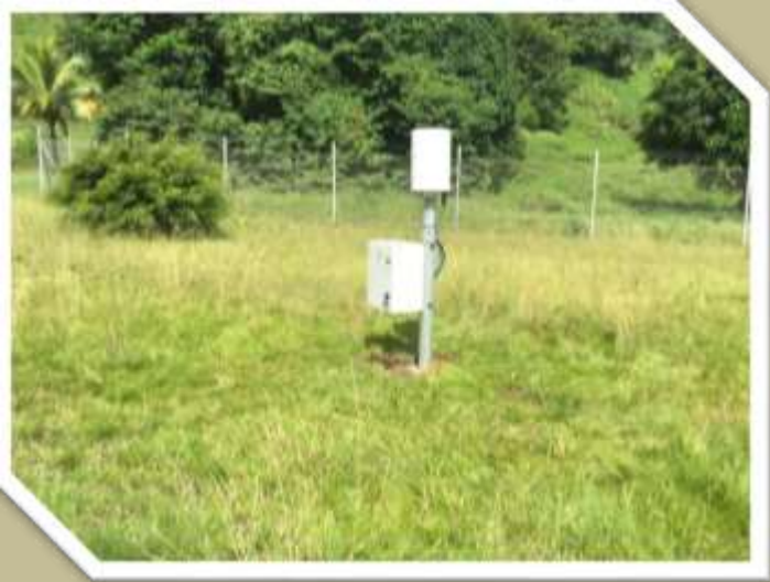
Automatic rainfall gauge installed in 2016 at Dalaway (Vermont St. Vincent and the Grenadines). Credit: CIMH
