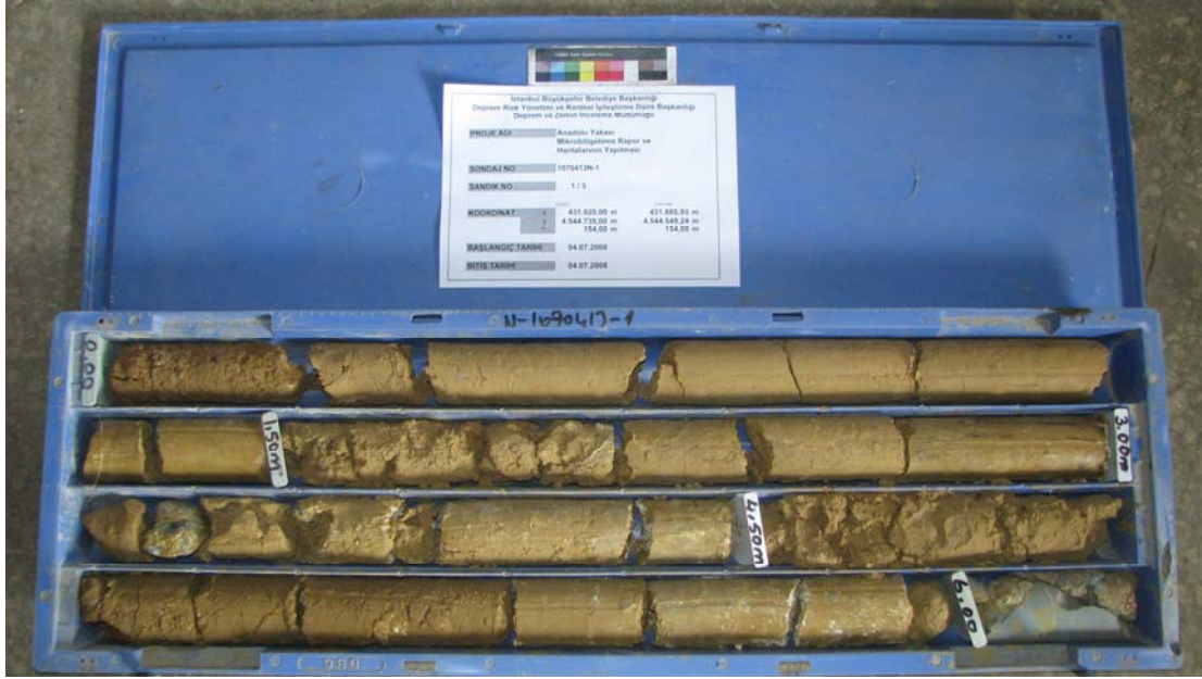
Figure 8.5 Core Chest ( Karstic clearance between 0 -6 m )
