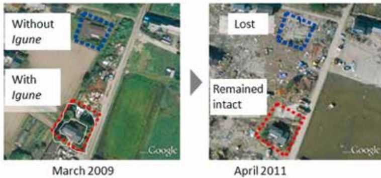
Figure 27. An example of a home that was not surrounded by an Igune and was later washed away by the tsunami (blue dashes) situated next to a home that was surrounded by Igune and was not damaged by the tsunami (red dashes). The white line shows the shape of the Igune . (Source: Ministry of Land, Infrastructure, Transport and Tourism, Japan, 2012)
