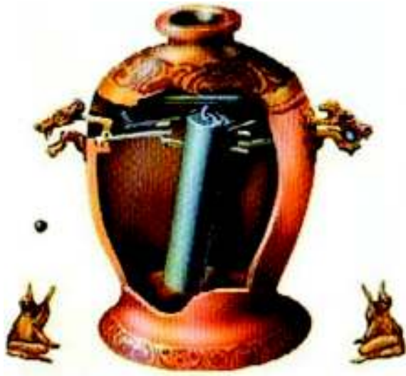
Figure 1. One of the historical earth quake detector (China, 2 nd Century).
