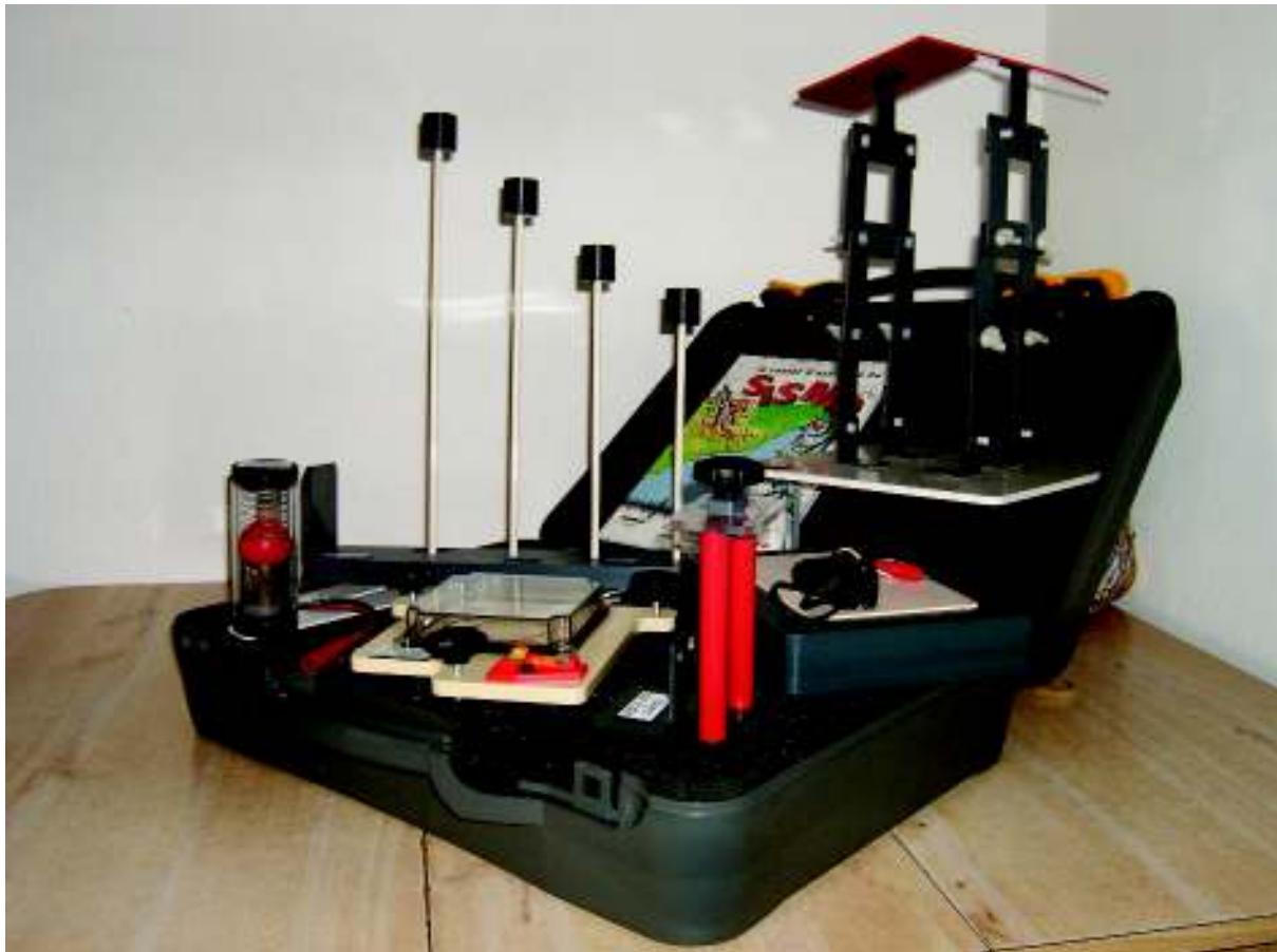
Toolkit for laboratory experiments by students: it has been designed during the NaRAs project for the illustration of different effect of seismic shaking.
