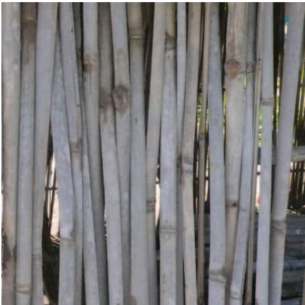
Bamboo - walls or lath to support mud
