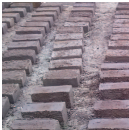
Mud blocks - construction of walls
