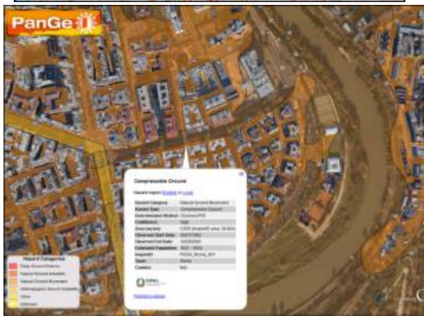
Figure 1C : Location of the project in relation to the Ground Stability Layer information which here indicates compressible ground associated with the fluvial deposits
