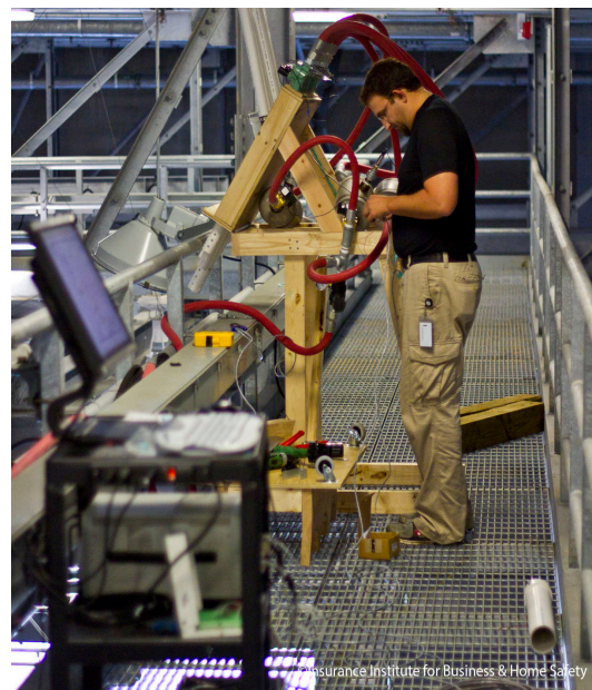
Dr. Ian Giammanco, IBHS research scientist, works on a hail cannon on the IBHS Research Center catwalk.
