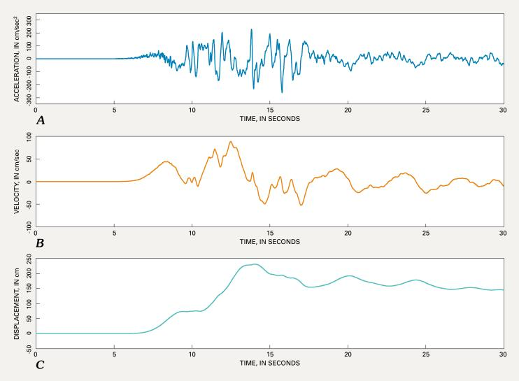
**Figure 4**. **A**, Recorded accelerations at the Kandilli Observatory and Earthquake Research Institute strong motion station, YPT, at the Petro-Chemical Plant in Korfez during the August 17, 1999, main shock. Station is about 4 km from the surface rupture. **B**, Velocities computed from acceleration time history showing large velocity pulse. **C**, Displacements computed for acceleration time history showing large displacement pulse. *Illustration by William L. Ellsworth.*
