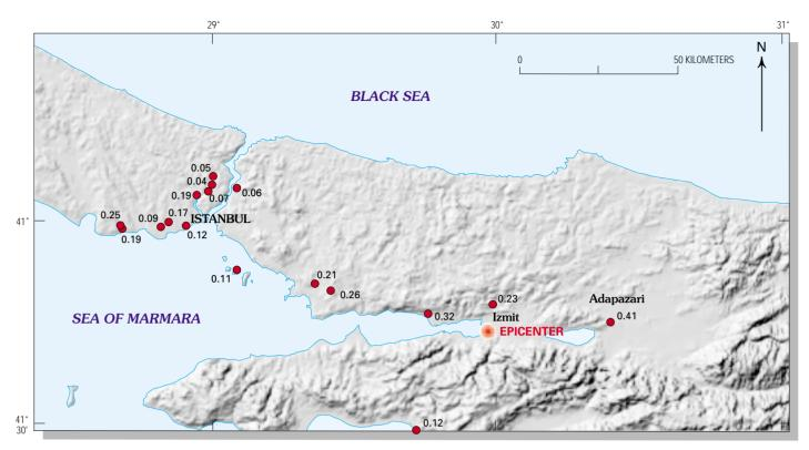
**Figure 22.** Map showing locations of peak horizontal accelerations recorded at strong motion stations in and near the epicentral area. The network stations included are from ERD, ITÜ, and KOERI. *Base map courtesy of BKS Surveys Ltd., N. Ireland.*
