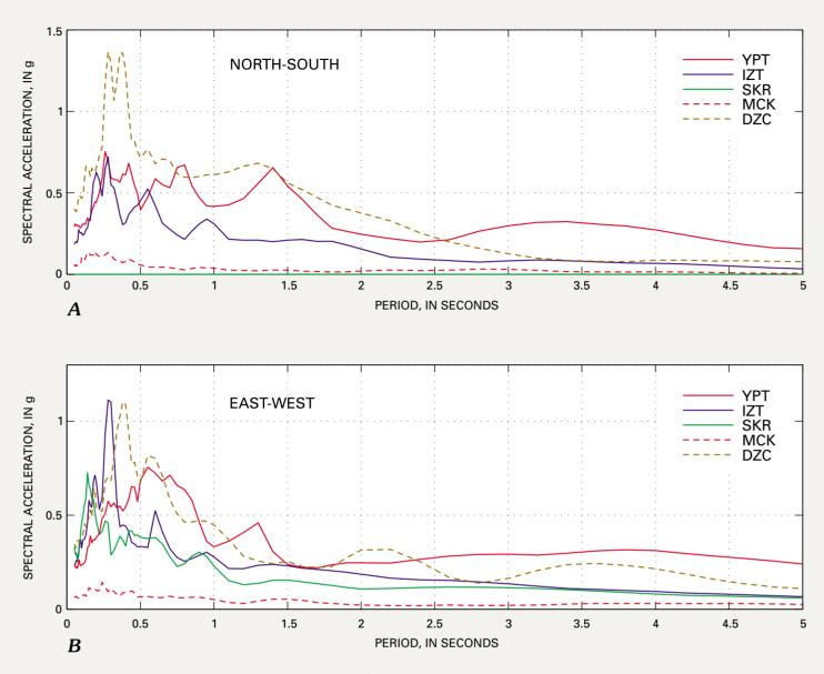
Figure 26. Actual pseudo-acceleration response spectra (A, B) and normalized (with respect to zero-period acceleration) response spectra (C, D) for 5 stations. The normalized response spectra also show the response spectra of the 1998 Turkish Building Code for stiff and alluvial soil site conditions. Illustration by Mehmet Çelebi.
