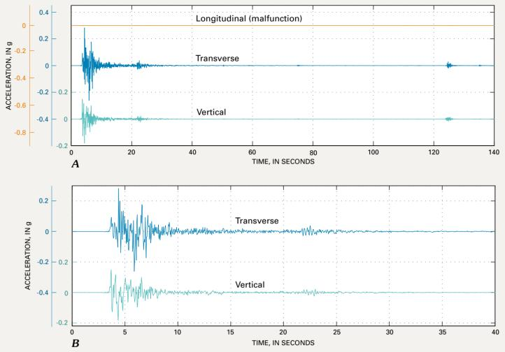
**Figure 23.** A, Time histories of acceleration for 140 s at SKR; note that longitudinal component malfunctioned. The plot shows several events: B, time history with first 40 s of the acceleration record; C, the cumulative sum of the squared acceleration values; and D, effective duration of significant strong motion during the main shock, based on time between 5 and 95 percentiles of the cumulative sum, is 4.5 s. *Illustration by Mehmet Çelebi*.
