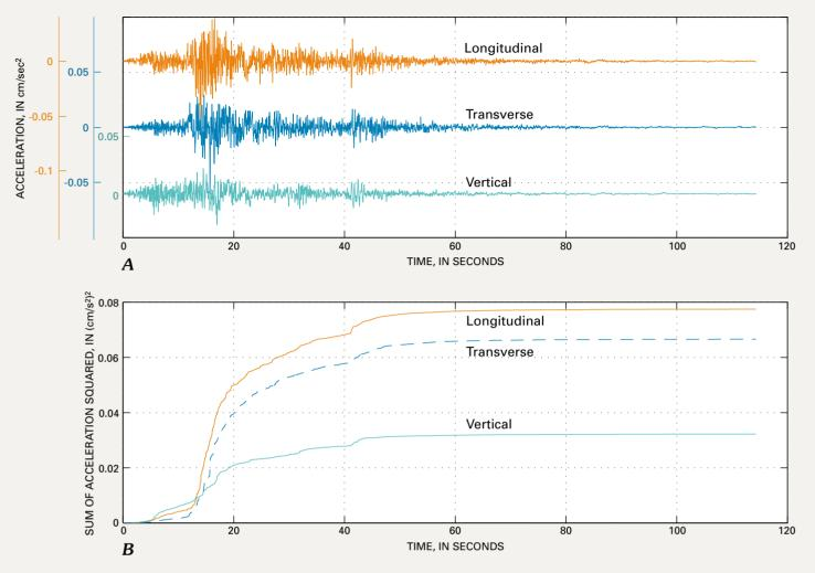
**Figure 25. A**, Time histories of acceleration at MCK in Istanbul. The plot shows several events. **B**, the cumulative sum of the squared acceleration values indicates the main shock contributed at least 90 percent of the total significant strong motion and the effective duration of strong motion was 36 s. *Illustration by Mehmet Çelebi*.
