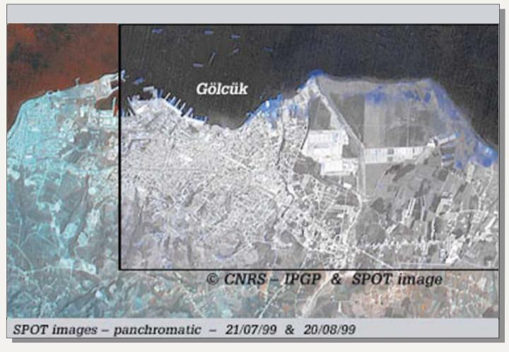
Figure 11. Satellite image of Gölcük area showing zones of coastal submergence (blue). Strike-slip faulting occurred through the port area (upper left) and oblique faulting occurred on the Gölcük (normal) fault. Copyrighted image by CNRS-IPGP and SPOT image; used with permission.
