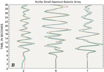
**Figure 32.** *A*, Pseudo-record section of ground motions from two pairs of stations at Dilovasi and Adapazari plotted on the same amplitude and time scales. Note the S-minus-P time of the first pair is approximately 5 s and that of the second is approximately 16 s. *B*, Overlay of Z, R, T components of closely spaced North, South, West stations at Korfez, all traces plotted on the same amplitude and time scales. *Illustration by Edward Cranswick*.
