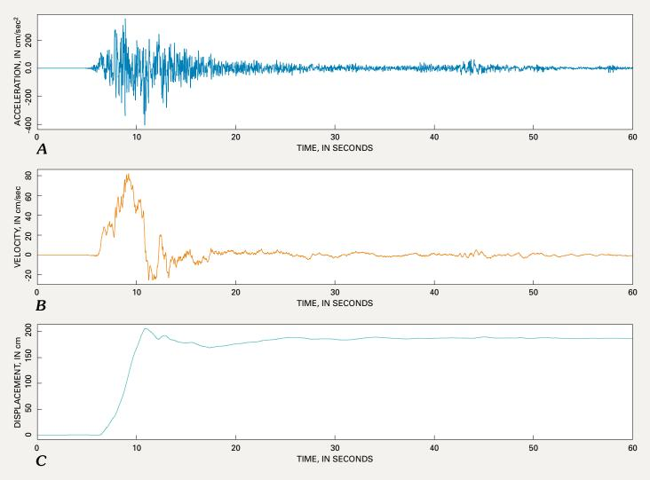
**Figure 3.** A, Recorded accelerations at the Turkish National Strong Motion Network station, SKR, in Adapazari during the August 17, 1999, main shock. Station is about 3.5 km from the surface rupture. **B**, Velocities computed from acceleration time history showing large velocity pulse. **C**, Displacements computed for acceleration time history showing large displacement pulse. **Illustration by William L. Ellsworth**.
