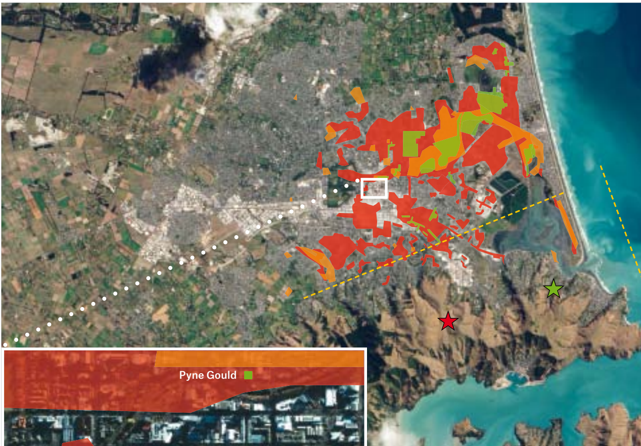
Areas in Christchurch (central business district enlarged) in which soil liquefaction was observed during the earthquakes on 4 September 2010, 22 February 2011 and 13 June 2011.
