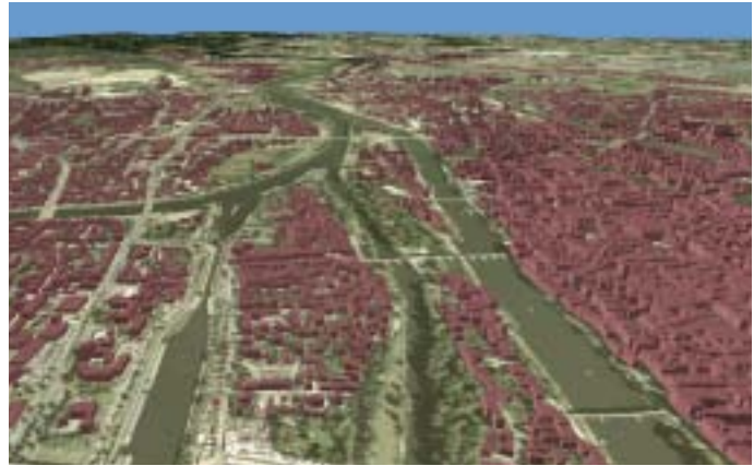
Three-dimensional building model (LoD1) of the city of Regensburg on the Danube.
