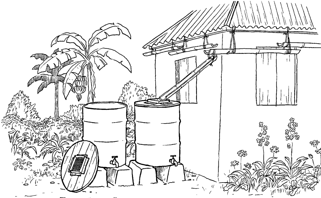
Using a tin roof to collect rainwater.
