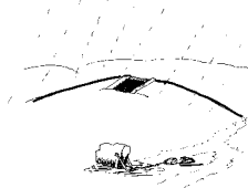
2. Mouth of hole built up to keep out runoff
