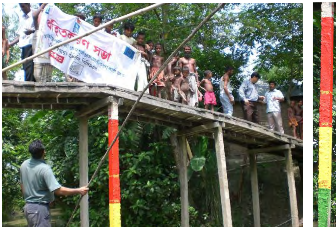
Figure 3-5. Community based flood warning system was set for pilot testing in selected sites.
