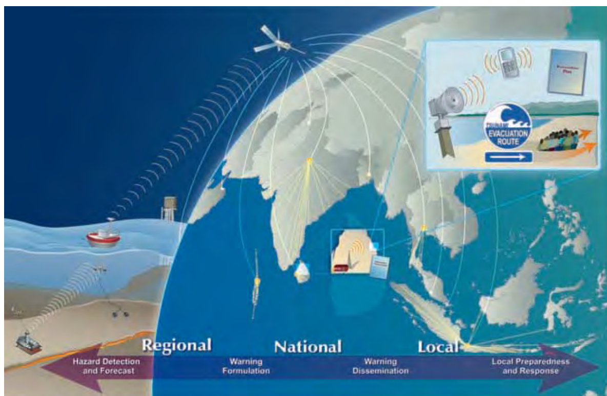
Figure 3-9. End-to-end tsunami detection, warning and preparedness process (Source: US IOTWS: 2008).
