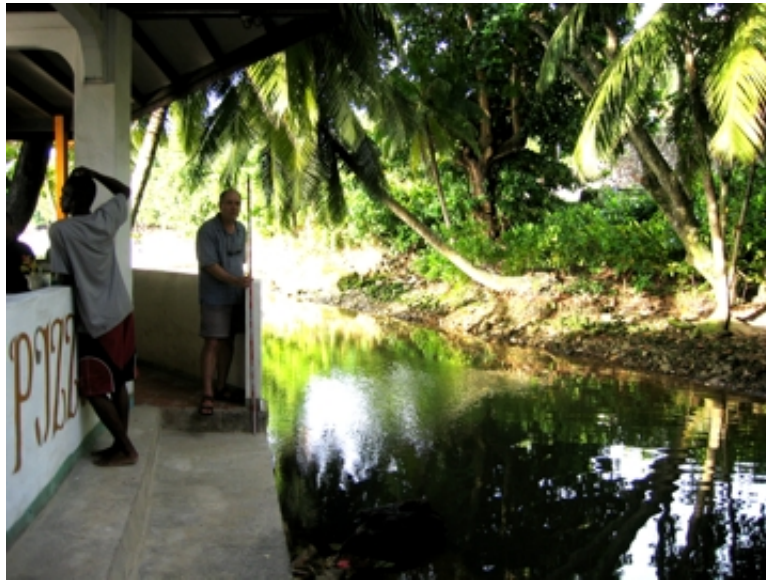
Fig. 53: Tsunami waters just reached the step upon which the two men are standing at Baobab Pizzeria, Beau Vallon. This is about 1.6 m above sea level shown in picture, or approximately at higher high tide level. Photo: LEJ (GSC), 23 Jan 2005.
