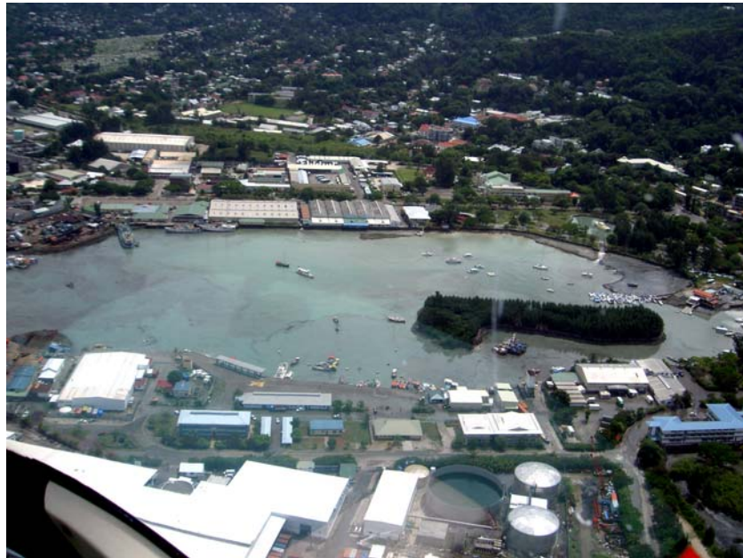
Fig. 9: Oblique aerial (looking south) view of the fishing harbour, from the north, 26 Dec 2004, during a low-water phase. The exact time of this photograph is not known, but the walls and paving on the fishing dock remain intact at this time. A fishing boat lies on its side to the left of the large white warehouse at lower left and some of the failure of the dock in that area may already have occurred. Photo courtesy of Dan Holtzhane.
