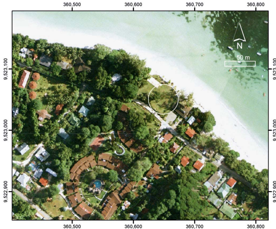
Fig 66: The Berjaya Praslin hotel complex. The grassy area immediately northwest of the pizzeria is circled. This area was flooded and received a tsunami deposit of well-sorted medium to fine sand (Figs. 67 - 69). The run-up in this area reached the seaward part of the semi-circular hotel complex. The limit is about 175 m from the top of the beach or about 200 m from the MSL shoreline.
