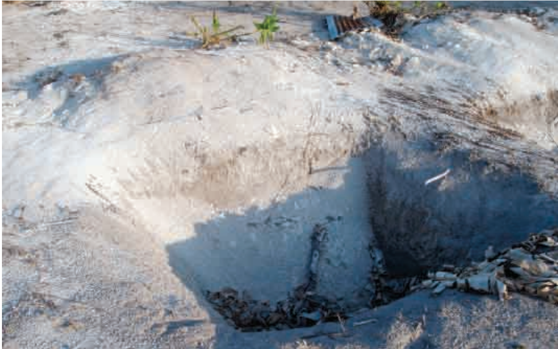
FIGURE 4.9: Sediment transport into banana pits on Kudakalhaidhoo Island. The wave came from the top left corner.
