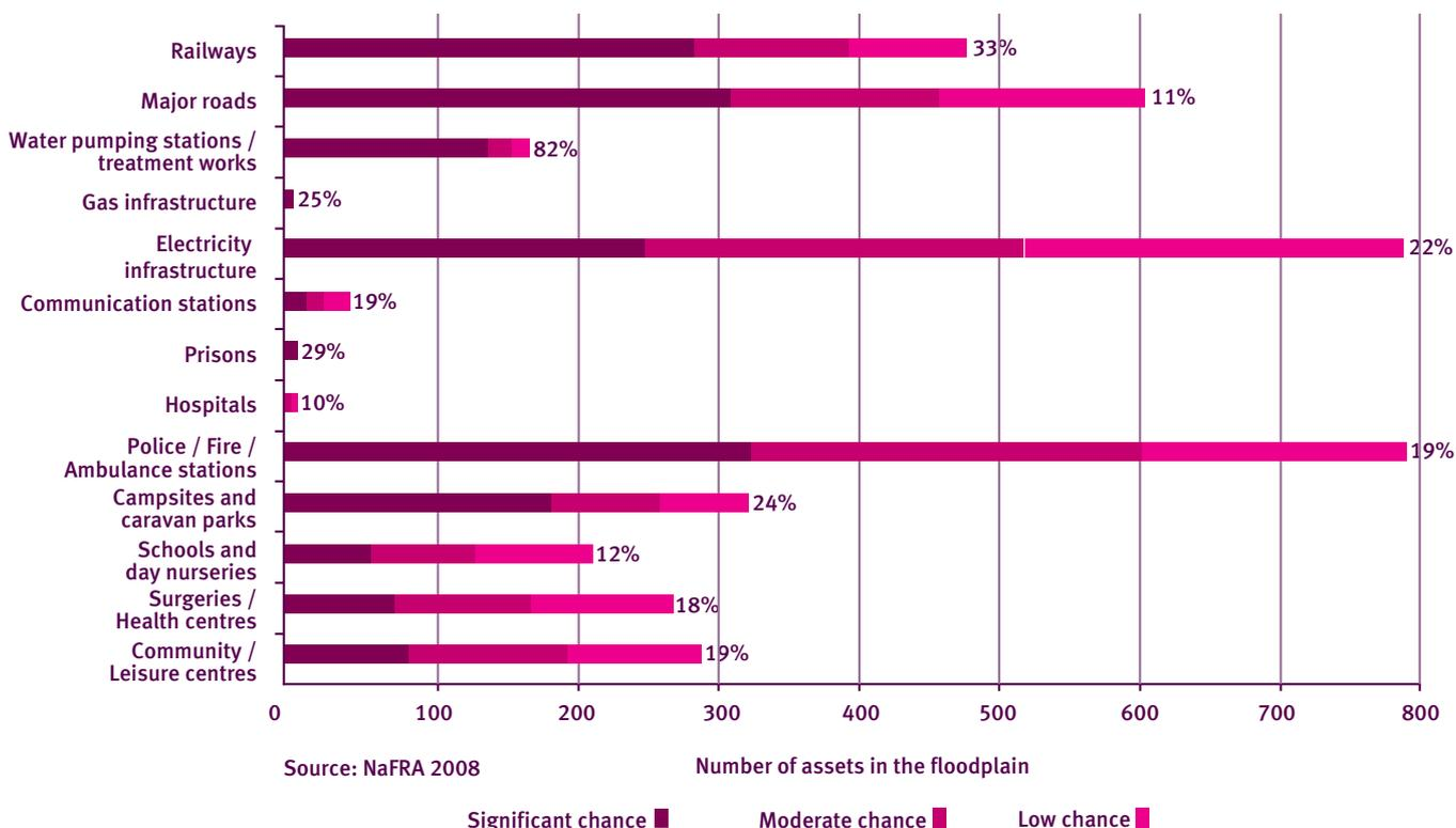
Water related infrastructure, such as water supply treatment works, pumping stations and sewage treatment works, is generally located close to rivers as their operation depends on access to the water. As a result more than 80% of pumping stations and water treatment works in Wales are in flood risk areas.
