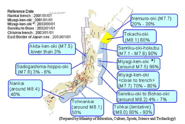
Figure A2.b - Probability of the occurrence of large earthquakes within 30 years.
