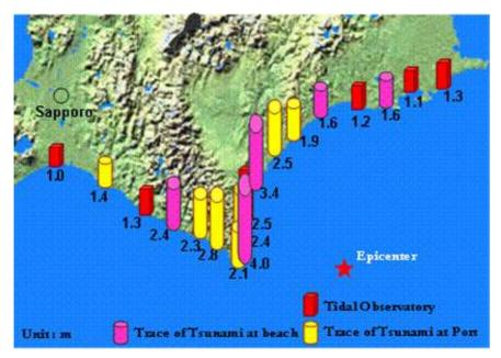
Figure A3.d - Distribution of tsunami height.
