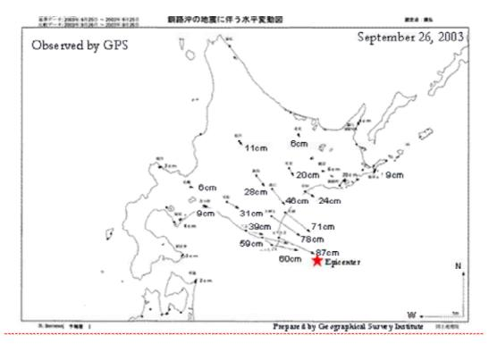
Figure A3.c - Horizontal displacement of crust.
