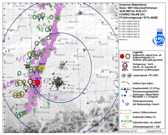
Figure B7.a – The KONRAD system forecasting the developments of an ongoing thunderstorm.
