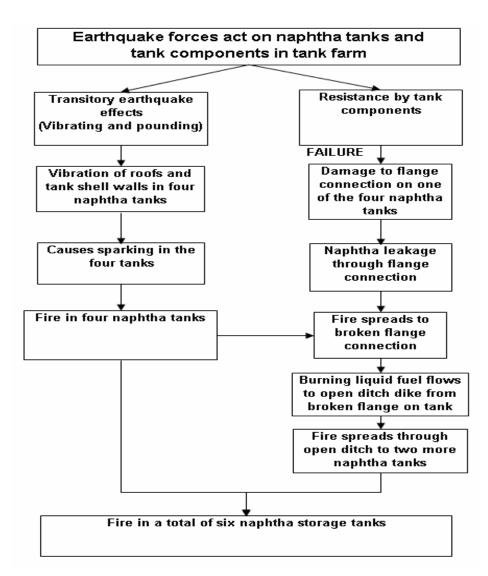
Figure A2.b - Earthquake triggered cascading events at the naphtha tank farm.
