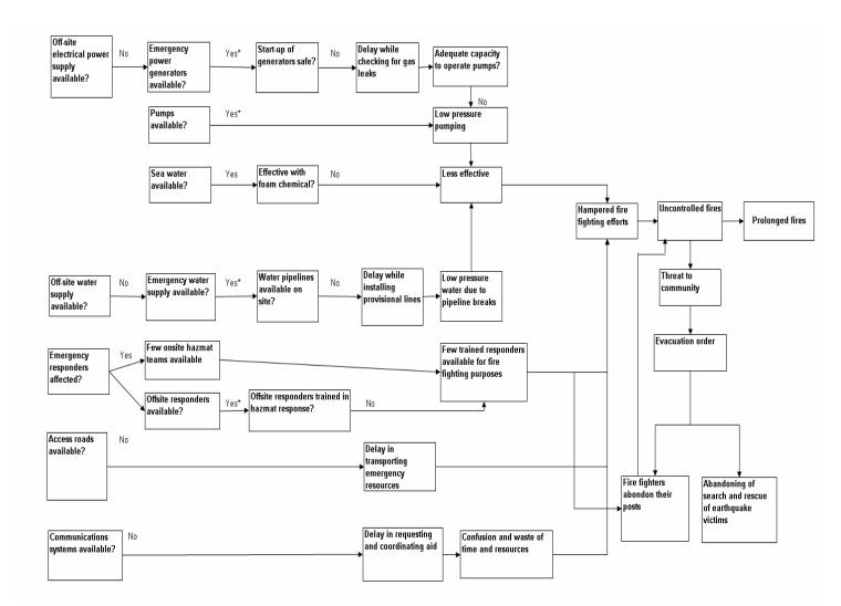
Figure A2.d - Cascading events which hampered emergency response to the multiple fires and hazmat release at an oil refinery following the Kocaeli earthquake.
