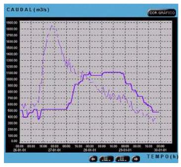
Figure B5.0 - Flood management in Aguieira dam: comparison between incoming and released flow.
