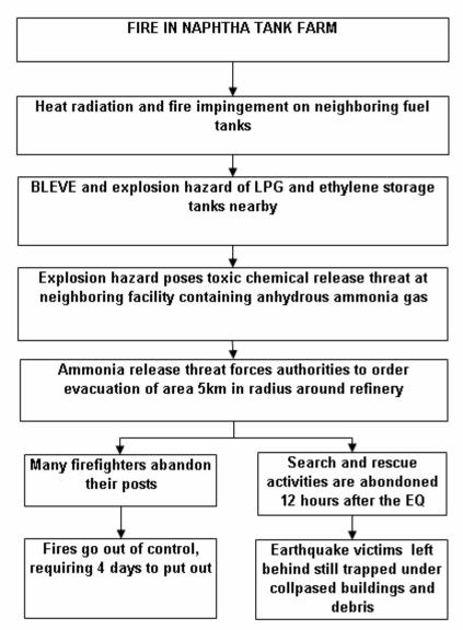
Figure A2.c - Offsite and onsite consequences of naphtha tank fires.
