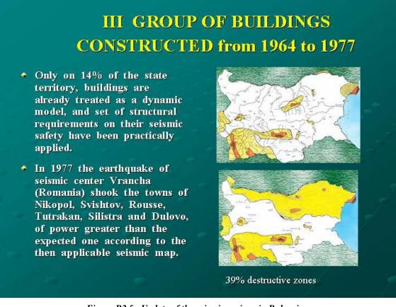
Figure B2.f – Update of the seismic regions in Bulgaria: destructive zones increased from 14% (map above) up to 39% (map below).
