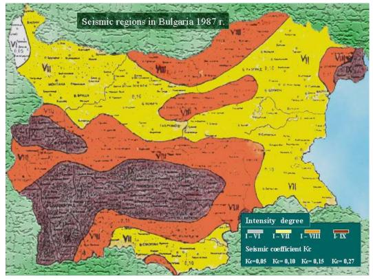
Figure B2.a - Map of seismic regions in Bulgaria, 1987.
