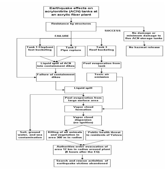
Figure A2.e - Earthquake effects on acrylonitrile storage tanks at the acrylic fibre plant.
