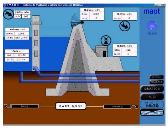
Figure B5.j - Information concerning dams, available in the Alert and Surveillance System for Water Resources.
