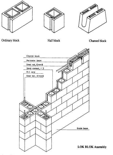
Case-study: Mortar-free interlocking blocks system (LOK BILD System)
