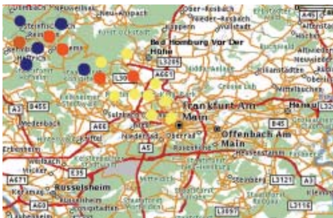
Fig. 2: Detail from a BLIDS product, showing the track of a thunderstorm and the distribution of lightning strikes. The bullets show the various lightning strengths. This kind of information can be used for the purposes of early warning and claims investigation ( www.blids.de ).
