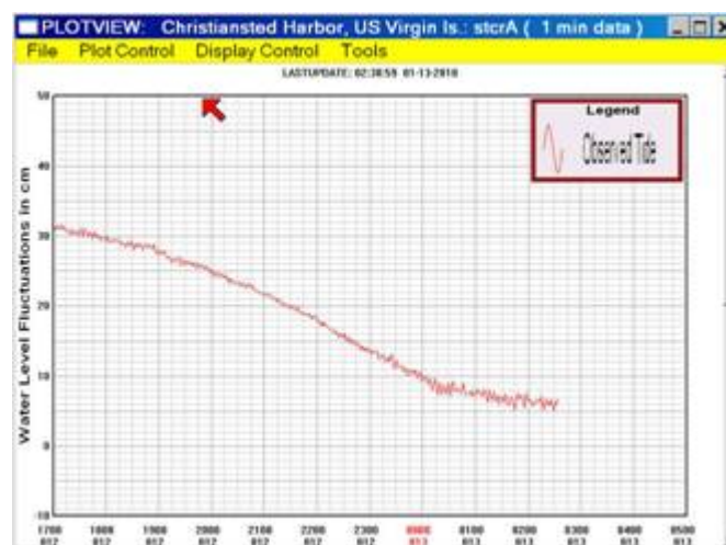
Figure 5. Tsunami record at Christiansted Harbor, US Virgin Island. The data sampling interval is 1 minute. Although tsunami record is not clear, tsunami arrival time will be around 23:25UTC.
