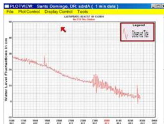
Figure 4. Tsunami record at Santo Domingo, Dominican Republic. The data sampling interval is 1 minute. The tsunami signal starts as a “rise” in sea level at 22:40 UTC and the amplitude of the oscillations gradually declined. The pulse around 2:30 UTC is noise.
