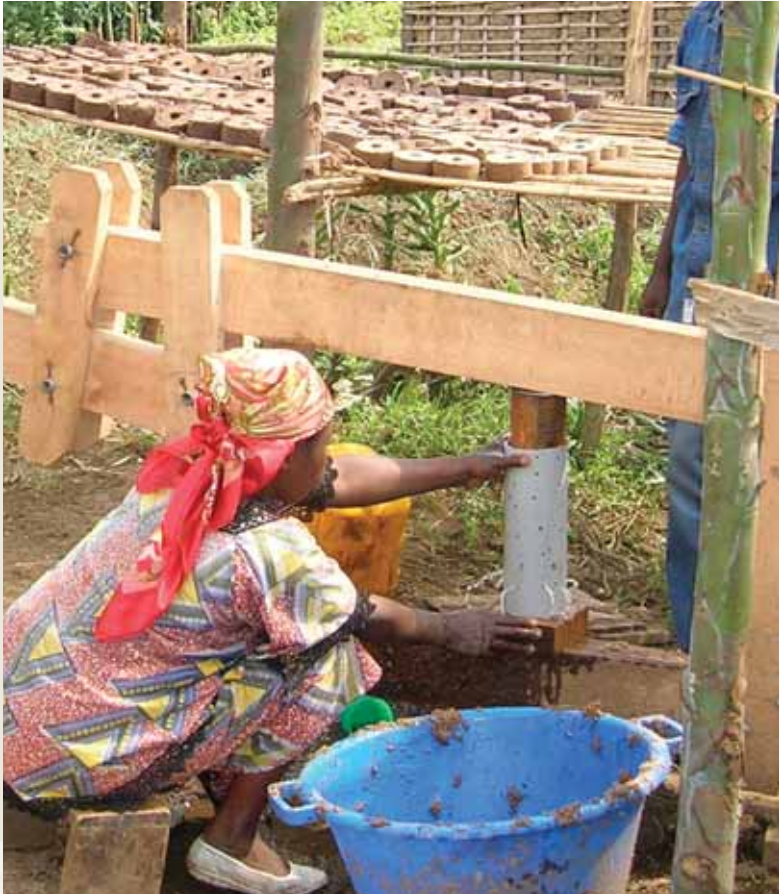
Production of fuel briquets at Kimumba village — an efficient and environmentally sound approach to providing fuel for cooking.
