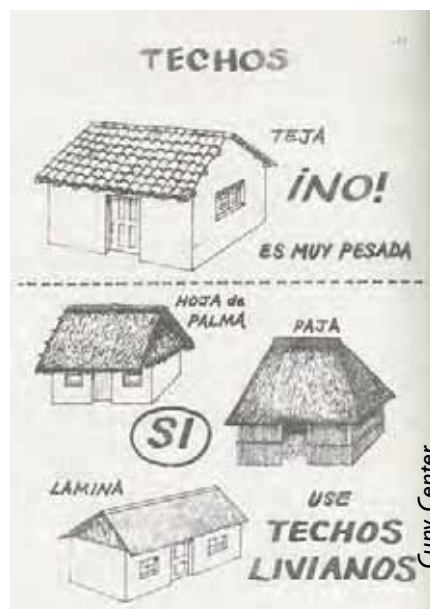
Options for roofing materials - tiles, palm leaves, thatch, corrugated iron
