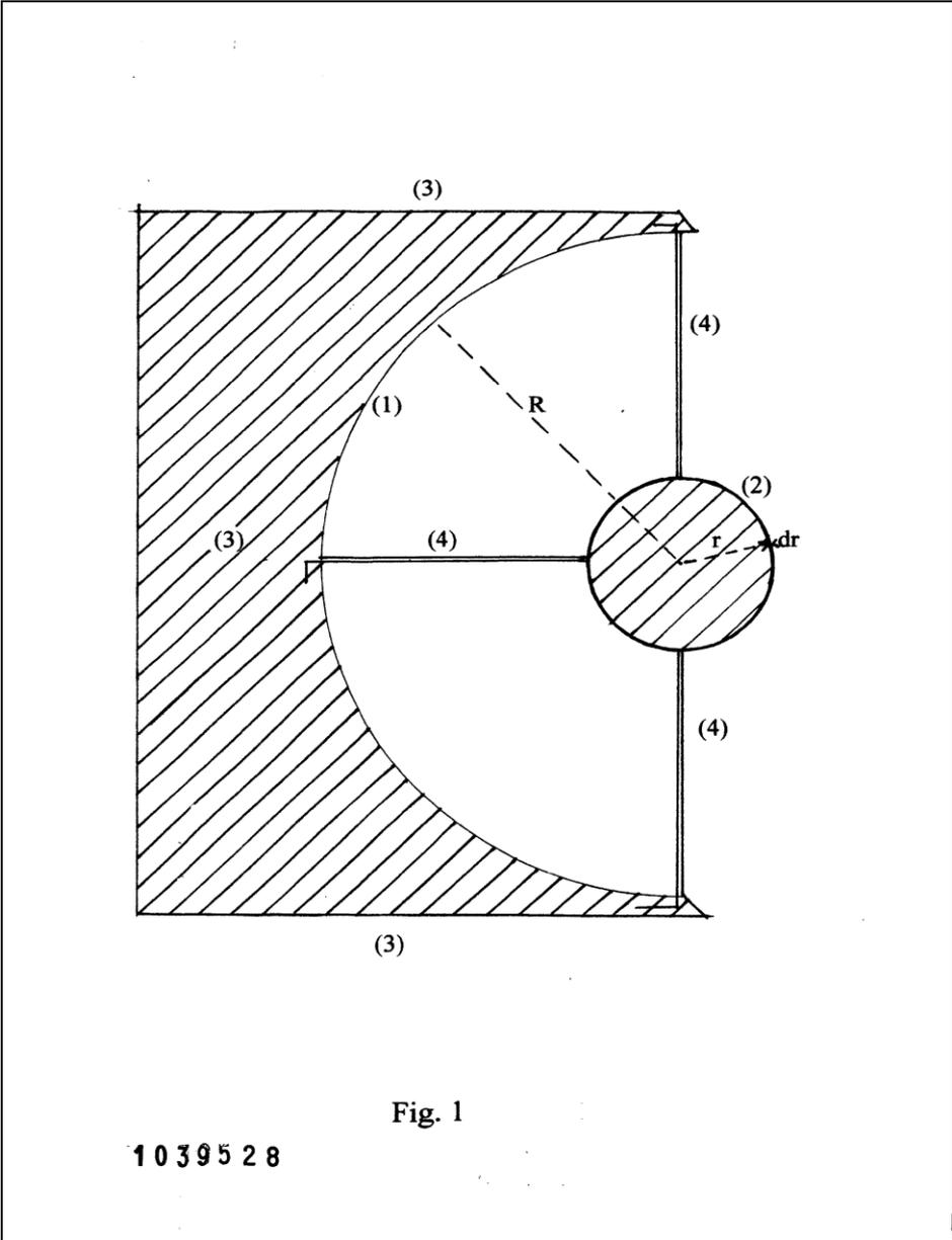
Figure 1: Vertical cross section of the return type breakwater or as horizontal cross section of the annihilation type breakwater, from patent NL 1039528 (EMID, 2013)
