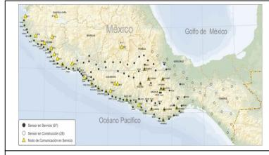
Figure 1. The solid black circles represent the distribution of sensing stations used in the Mexican Seismic Alert System. (source: CIRES, Mexico)
