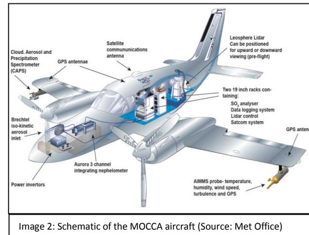
Image 2: Schematic of the MOCCA aircraft (Source: Met Office)
