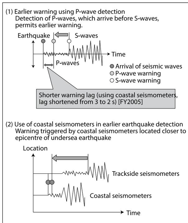
**Figure 1:** Diagrams showing the additional seconds of warning time given by improved detection of P-waves and use of coastal seismometers. *Source: Ogura, 2006<sup>9</sup>.*
