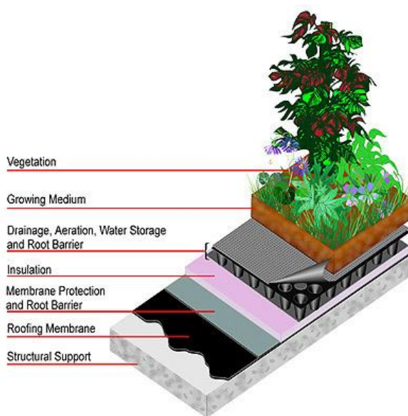
Figure 7: Typical Green Roof
