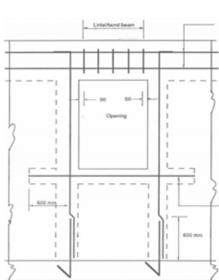
Figure 56: Reinforcement details around openings in walls
