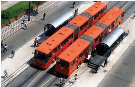
Figure 3.8 Bi-articulated BRT Bus and Bus Station Source: IPPUC
