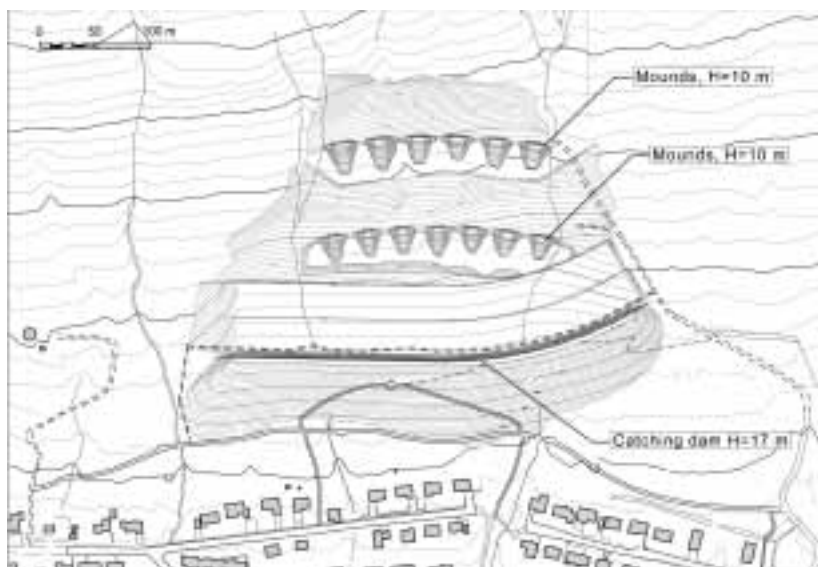
Figure 15.7: Plan view of combined braking mounds and a catching dam, made from reinforced earth. Neskaupstaður, eastern Iceland (designed by VST Consulting Engineers Ltd. and Forverk Consulting Engineers Ltd. in Reykjavík, Iceland, and Cemagref in Grenoble, France).
